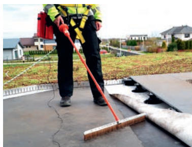
TROCKENORTUNG: HIGH VOLTAGE – SENSOR LEAK DETECTION
