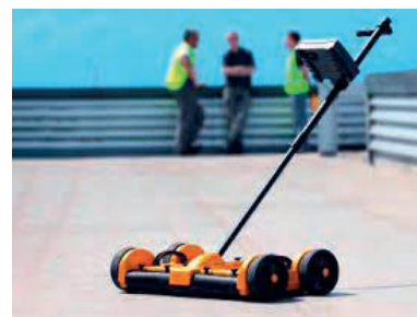
FEUCHTEMESSUNG: IMPEDANCE – SENSOR LEAK DETECTION
